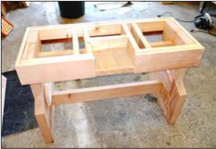
Left: A shelf is added in the back of the table for a book or small cup for water. Right: A front view of just the completed table base assembly.
