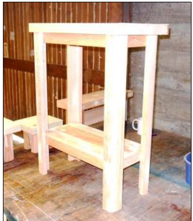
Front & side views of yet another stand or table--27" tall, with a 22" by 12" top.
