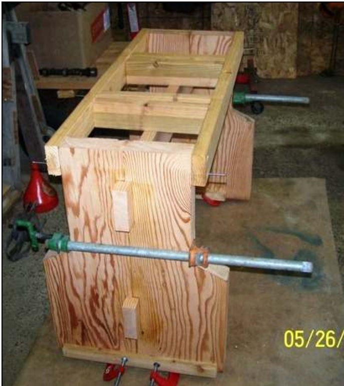
Left: Length members are added to the tops of the legs to hold the support cross pieces that also attach the table top. Right: Jeff runs boards for the table top cross pieces through the jointer to make a clean surface to attach to the underside of the table top.
