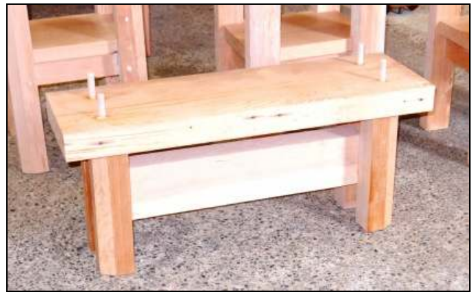
Left: The bases for the matching two short stands, to go with the tops shown above. These stands, when fully assembled, will be 12" tall. Right: Another stand, 9" tall, with its top installed and ready to sand.
