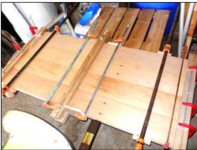
The table top—28" x 60", tied together with dowels and lots of glue and clamps Lots of planing, jointing, drilling out holes for dowels, gluing, and filling old holes!
