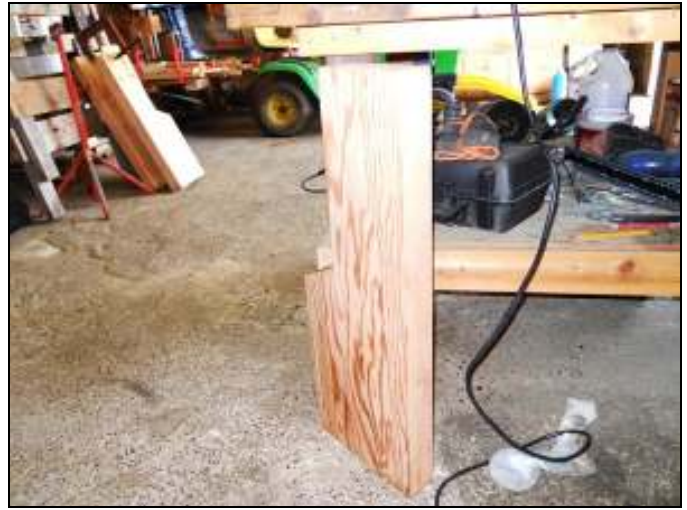
Planing and jointing--the legs after this process. Left: Outside view of one of the legs Right: End view of one of the legs
