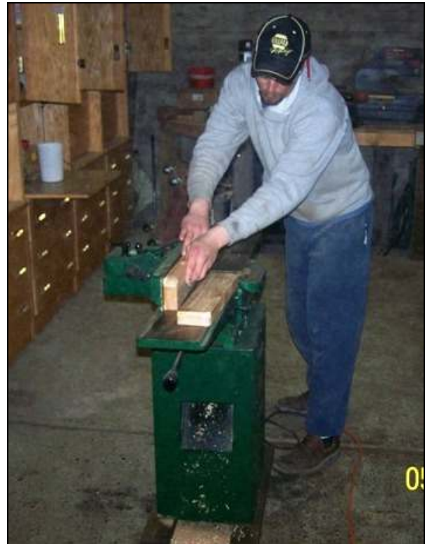
Left: Length members are added to the tops of the legs to hold the support cross pieces that also attach the table top. Right: Jeff runs boards for the table top cross pieces through the jointer to make a clean surface to attach to the underside of the table top.
