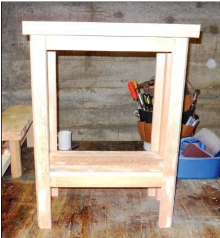
Front & side views of yet another stand or table--27" tall, with a 22" by 12" top.
