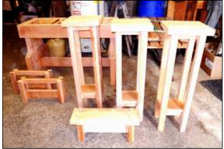
Left: More stands top were each built from two pieces, heavily glued and clamped to dry overnight. These 2 tops are 21" long, 7" wide, and about 1 1/2" thick. Once dried, they can be sanded and attached to the bases. Right: The collection of all of the assembled flower/candle stands—tall & short.
