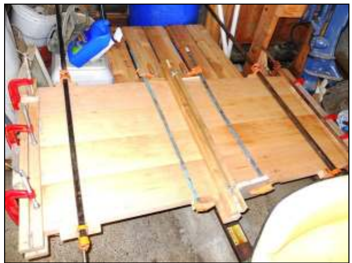
The table top—28" x 60", tied together with dowels and lots of glue and clamps Lots of planing, jointing, drilling out holes for dowels, gluing, and filling old holes!
