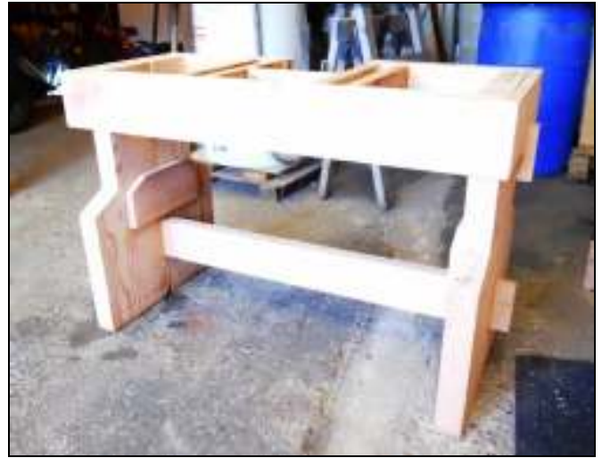
Left: A shelf is added in the back of the table for a book or small cup for water. Right: A front view of just the completed table base assembly.
