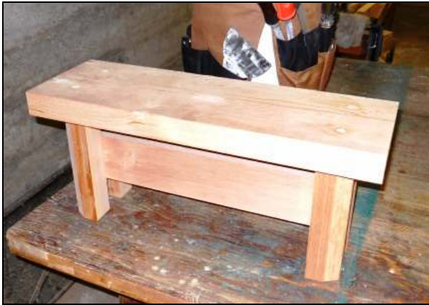
Left: 9" tall stand, with its top installed, dowels cut, and ready to sand. Right: a 12" tall stand, ready to sand.
