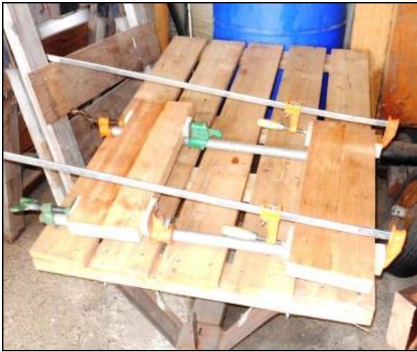
Left: More stands top were each built from two pieces, heavily glued and clamped to dry overnight. These 2 tops are 21" long, 7" wide, and about 1 1/2" thick. Once dried, they can be sanded and attached to the bases. Right: The collection of all of the assembled flower/candle stands—tall & short.
