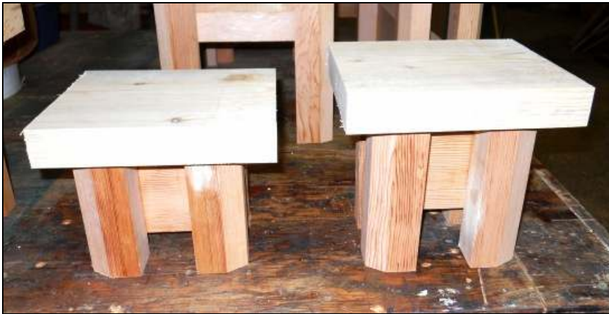
Left: 9" tall stand, with its top installed, dowels cut, and ready to sand. Right: a 12" tall stand, ready to sand.
