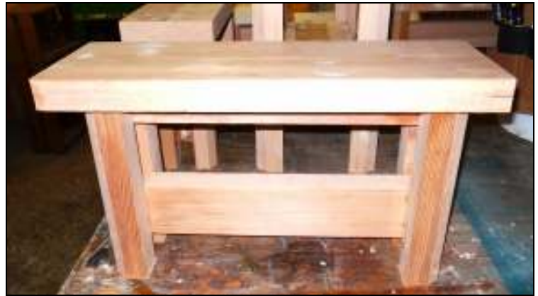
Left: 9" tall stand, with its top installed, dowels cut, and ready to sand. Right: a 12" tall stand, ready to sand.
